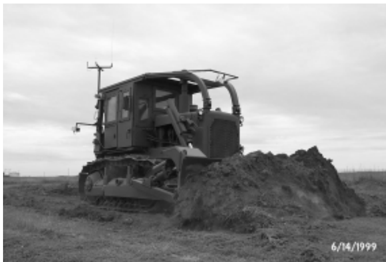
Figure 2: Caterpillar D7 Bulldozer
